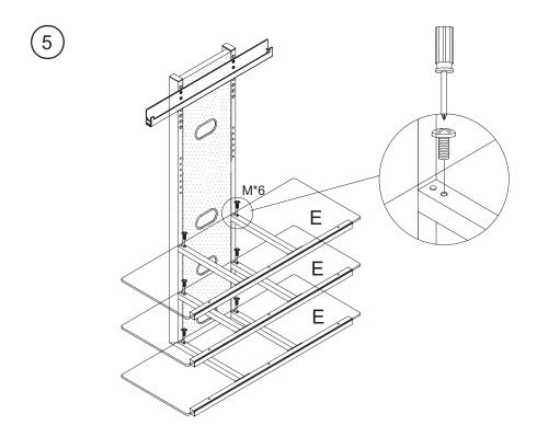
5-Fasten the glass (E) on the beams with screws (M). Do not over tighten screws.
